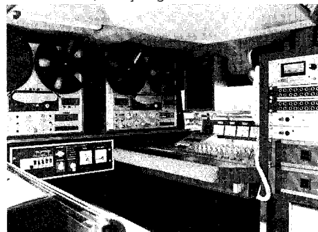
Interior audio equipment (l.t.r. below): Mains voltage supply, mixing console 269, rack with limiter jackfield, amplifier, transmitter (l.t.r. above) PR 99 tape recorders, air conditioning, loudspeakers, TV monitor, monitoring receiver.
